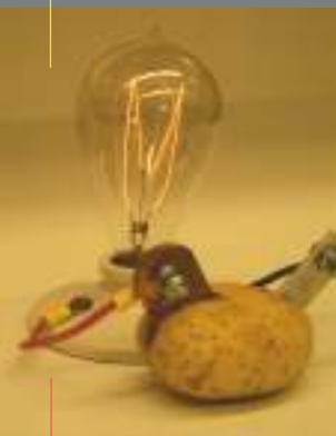
Potato Power - potato as a battery, used to power a lightbulb.
